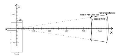
Standard Models of the ZLDS210 scanner can be de-livered in 8 different measuring ranges, and each in two versions with different measuring angles, either 10° or 50° and then in 2 or 3 scan rates giving high or low angular resolution, and can furthermore be customized to other than standard scan angels and measuring ranges.
